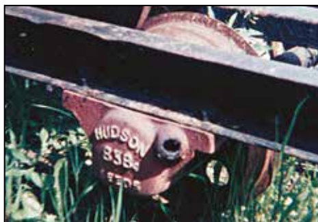
The maker's identity "Hudson 838 Leeds" cast into the axle bearing plate of one of the waggons.
