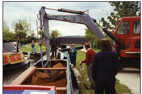
John Baylis unloads the crushed brick with the Ruston 3RB at Langley Mill before the rally.
