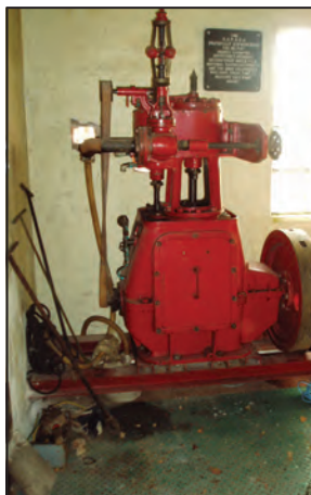
Single-cylinder steam engine from Shipstone's Brewery. Made by Matthew Paul & Co, Levenford Works, Dumbarton, engine number 5864.
