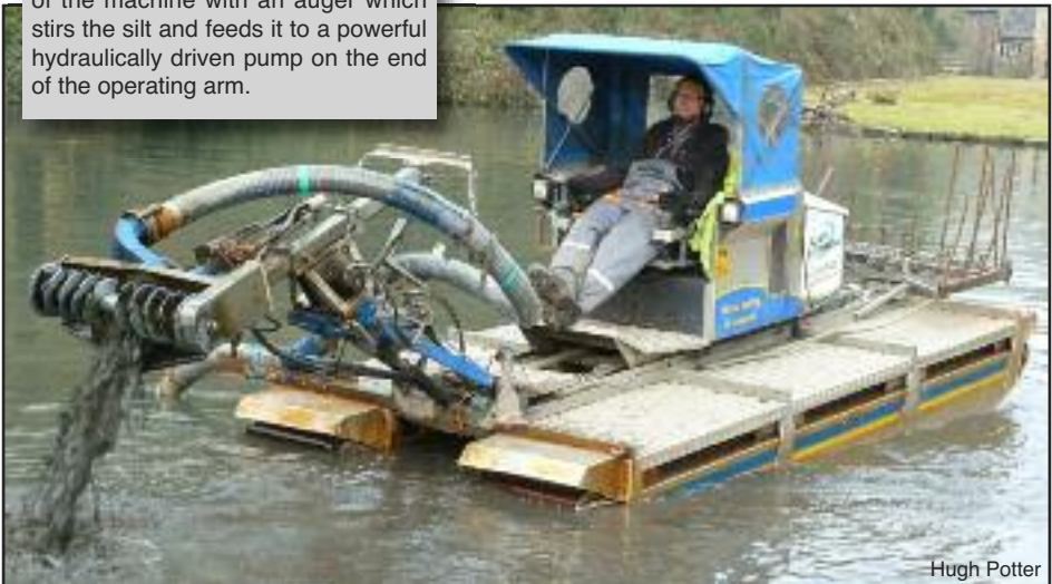
ABOVE: The amphibious dredger is simply driven from the field into the canal to start work.
